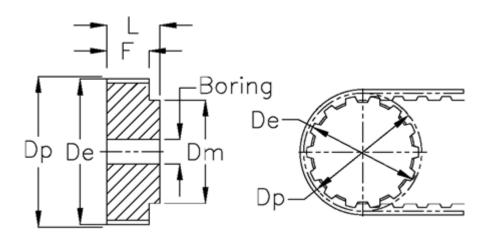
Type = T10Belt width = - 50 mm Weight = 2.42= 138.2De Dm = 88 = 140.2Dp F = 56 L = 66 Pre-drilled = 16 Tooth number = 44
